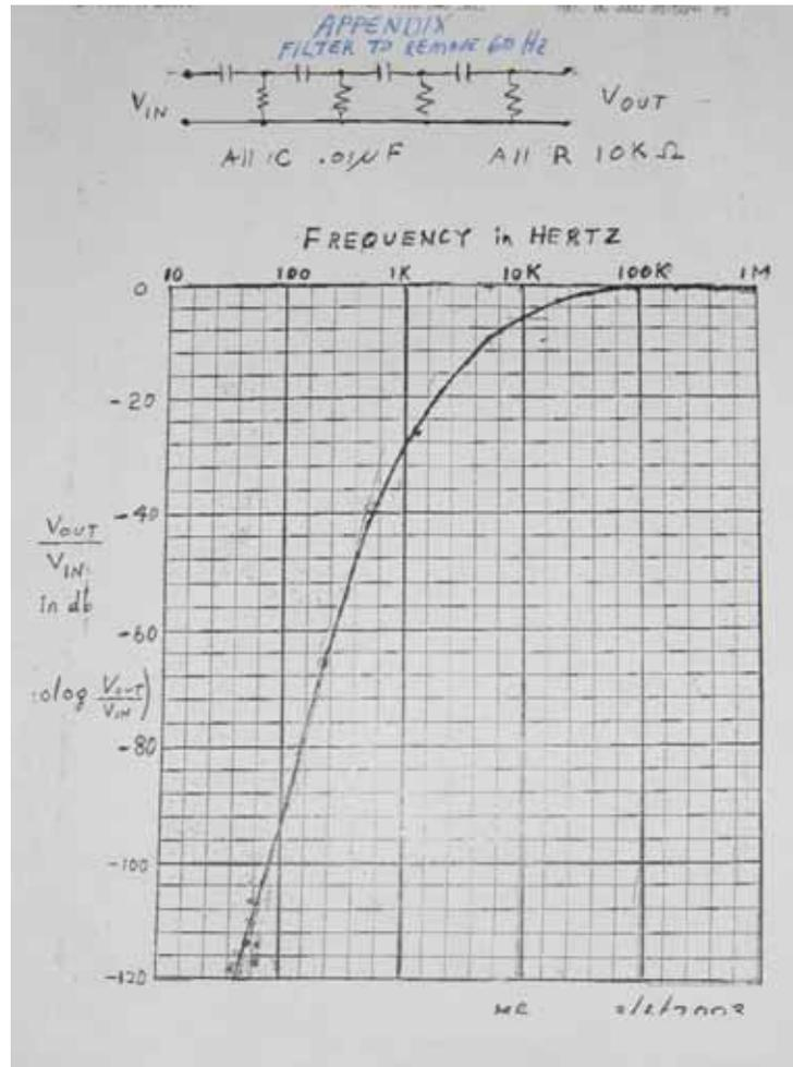
The filter in Figure One has the effect of reducing the amplitude of all frequencies below 10 kHz. The curve shows the attenuation in db, decibels, (Y-axis) with frequency in Hertz (X-axis). For non-electrical engineers the following translation is appropriate:
